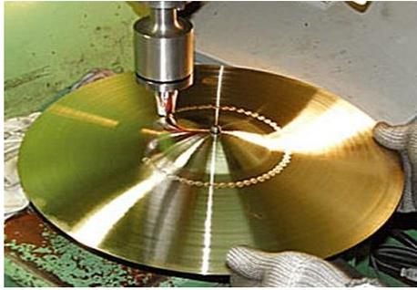
Fig. 2 Hammering process.
